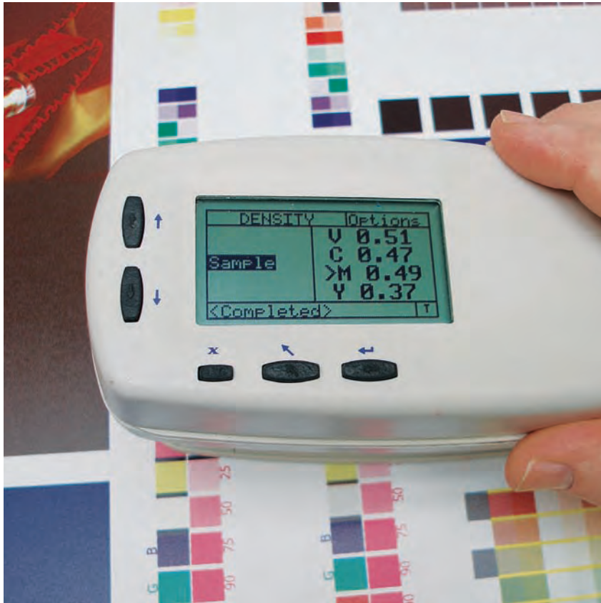
The G7 methodology still involves measuring colours with a spectrophotometer, which means first learning and understanding the L*a*b* colour space.
