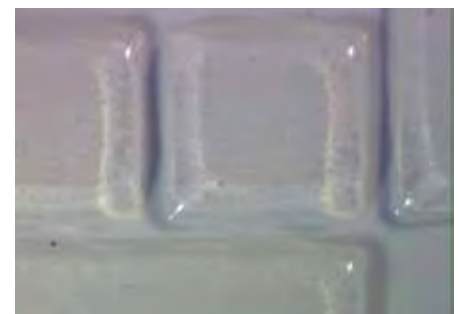
Figure 10: A top-down view showing a square printed into a white substrate.
