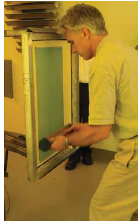
Figure 4: A screen coated from the square side of the screen.
