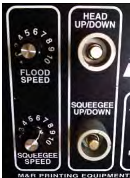
Figure 6: Printing press set with a slow flood bar speed and a fast squeegee speed.
