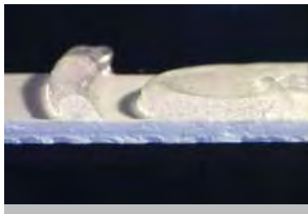
Figure 2: A grid view of a printed image cut through the substrate and ink film.
