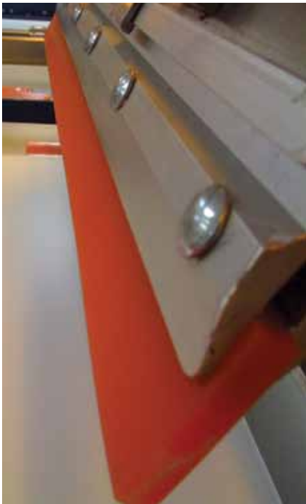
Figure 5: Squeegee with a lower angle setting.
