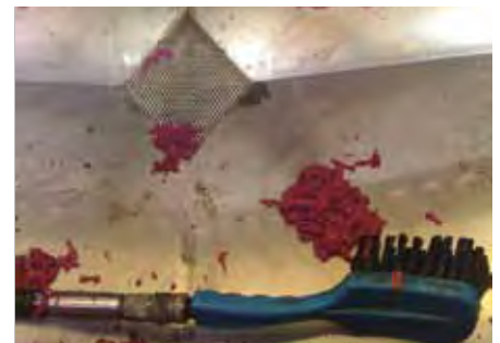
Figure 9: A view of the bottom of the reclaiming sink. The chunks of un-dissolved emulsion were filtered before going into the drain.
