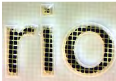
Figure 3: Thick stencil using clear emulsion, photo-film and an 8k metal-halide lamp. Photo courtesy of KIWO.
